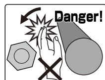
⑤ After tightening operation, it is often hard to detach the wrench because elastic force generated inside of the wrench is imposing a large load in between reaction arm and bolt/nut. After tightening operation, it is often hard to detach the wrench because elastic force generated inside of the wrench is imposing a large load in between reaction arm and bolt/nut. In such case, execute following procedure to release load to detach the wrench.
