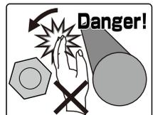
⑤ After tightening operation, it is often hard to detach the wrench because elastic force generated inside of the wrench is imposing a large load in between reaction arm and bolt/nut. After tightening operation, it is often hard to detach the wrench because elastic force generated inside of the wrench is imposing a large load in between reaction arm and bolt/nut. In such case, execute following procedure to release load to detach the wrench.
